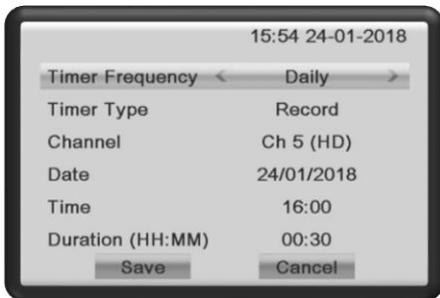
The Timer Setting menu allows you to set the viewing or recording schedule. A total of 32 timers may be set. Each timer includes the following settings.
